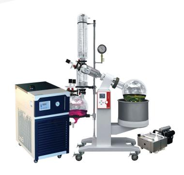
Rotary evaporators are used in chemical laboratories for the efficient and gentle removal of solvents from samples by evaporation. Rotary evaporation is most often and conveniently applied to separate "low boiling" solvents such a n-hexane or ethyl acetate from compounds which are solid at room temperature and pressure.
